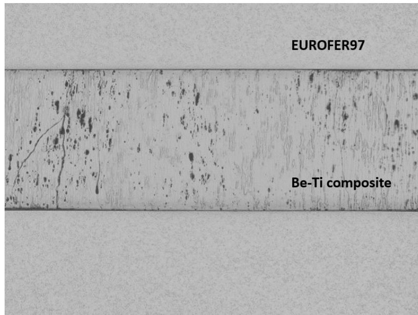
Figure 7. Microstructure of contact zone of Be-Ti composite and EUROFER97 after compression test at 700°C, 10MPa (500N), 200 h. (OM)
