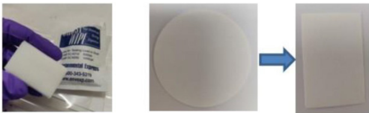
Figure 2.7: Folded Ghost Wipes (left), Whatman n°1 filter paper (centre), cut Whatman n°1 filter paper (right)
