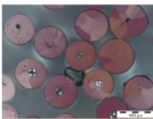
Microstructure of Be pebbles
