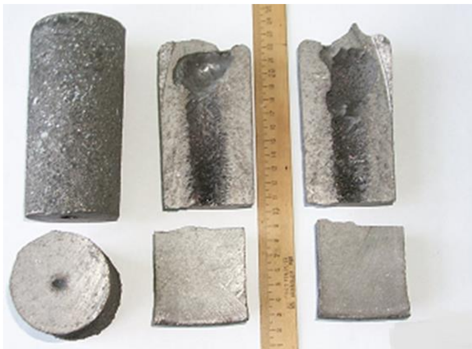
Figure 1. Ingots of titanium beryllide with casting defects.
