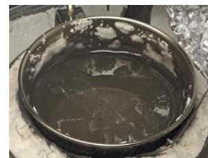
Below: melted FLiBe in a pot before purification.
